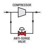
MOGAS anti-surge valves can withstand high temperatures, high pressures, corrosive applications, abrasive particulates, acidic products, lethal media and other critical conditions.
