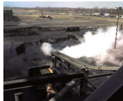
The lockhopper builds pressure as the reaction occurs, and then discharges the byproduct—water with 17% weight slag slurry—to a collection pit for collection and removal.
