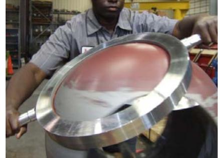
*The sealing surfaces are wide and in full contact with the surface of the ball 100% after the final mate lapping operation.*
