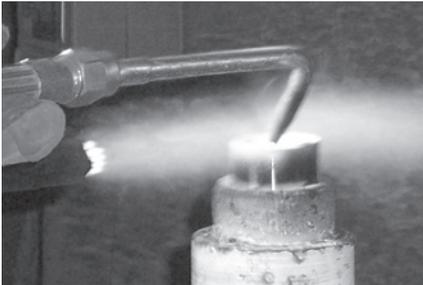
*Using the latest technology, this seat is receiving a coating. MOGAS coatings are specially chosen to handle the operating conditions of each application.*
