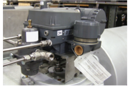
The smart positioner receives feedback of the valve travel position. This allows the instrument to diagnose the valve and actuator to which it is mounted – providing cost effective, preventative maintenance information.
